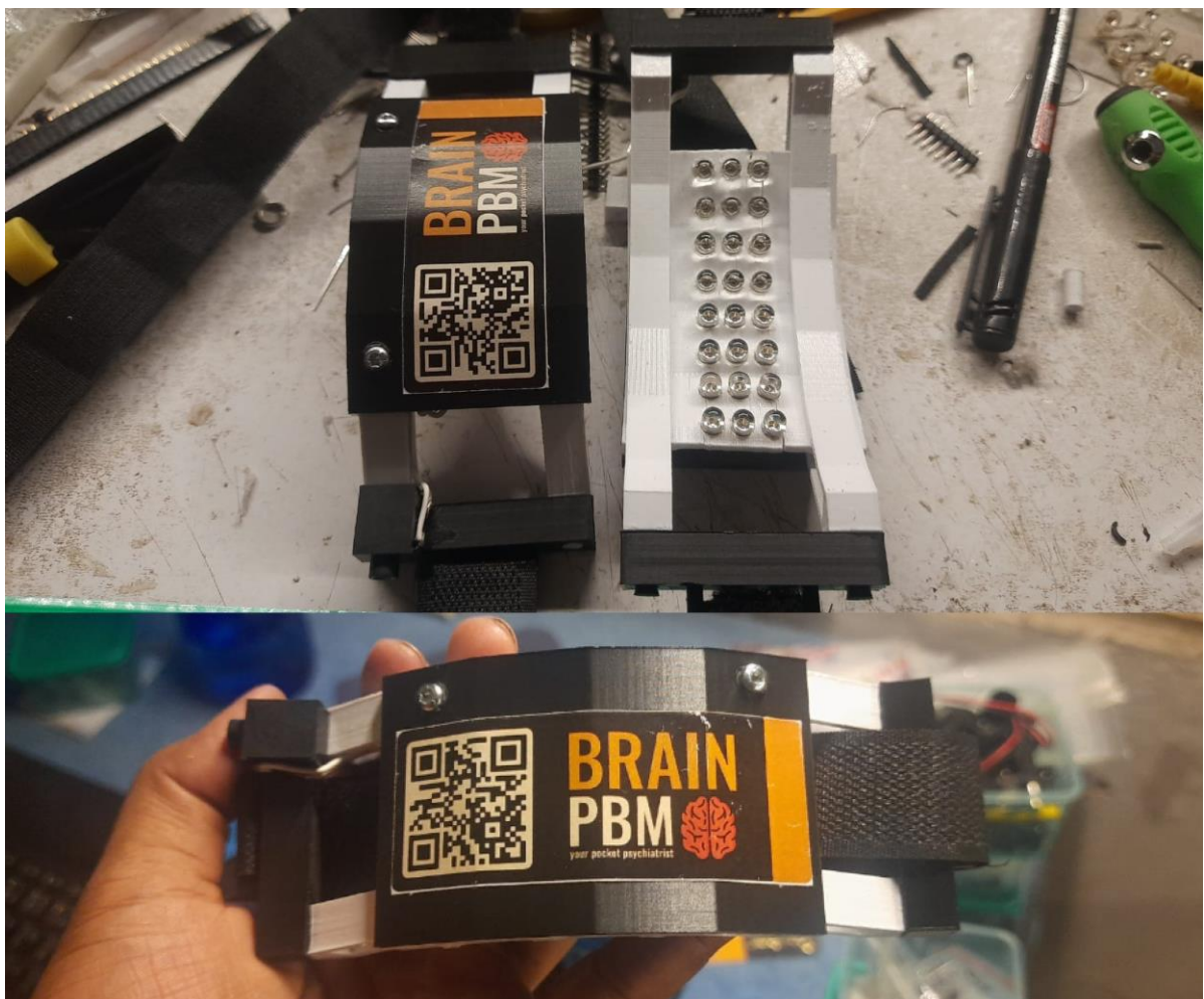
Figure 25: completely mounted and assembled head unit (top), size of head unit compared to the palm (bottom)
